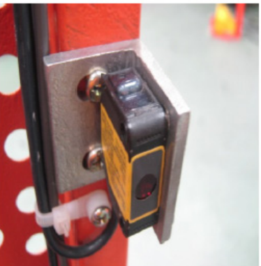
Receiver - No lights on. Indicates no power supply.
